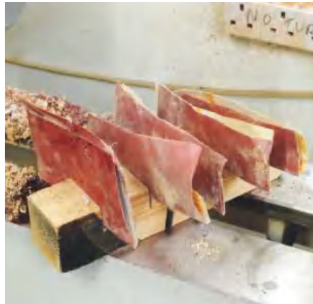
STEP 32. This little abrasive holder is great for keeping everything in order when working through the different grades of abrasive – picking up one in the wrong order will often mean that you have to start again
